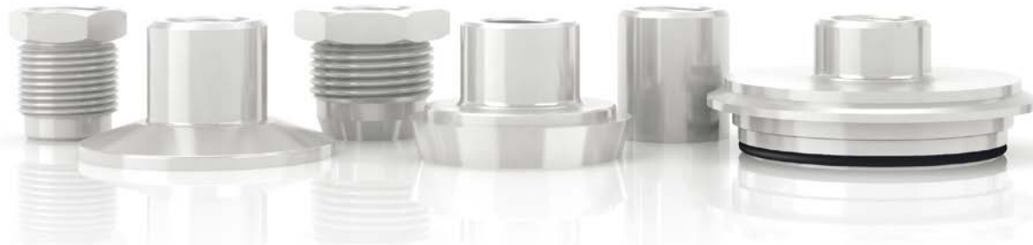
The modular process connection of USG 20 uses an adapter system which covers all standard process connections. All it takes to adapt the level switch to the process is to screw on the required connection.
